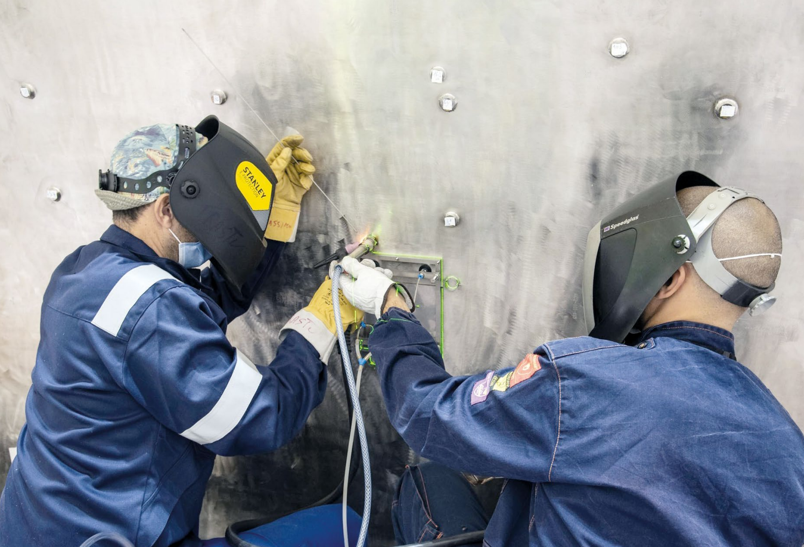
Fig. 1: The laser is projecting welds and laser contours precisely and directly onto the component, photo: ITER Organization.
