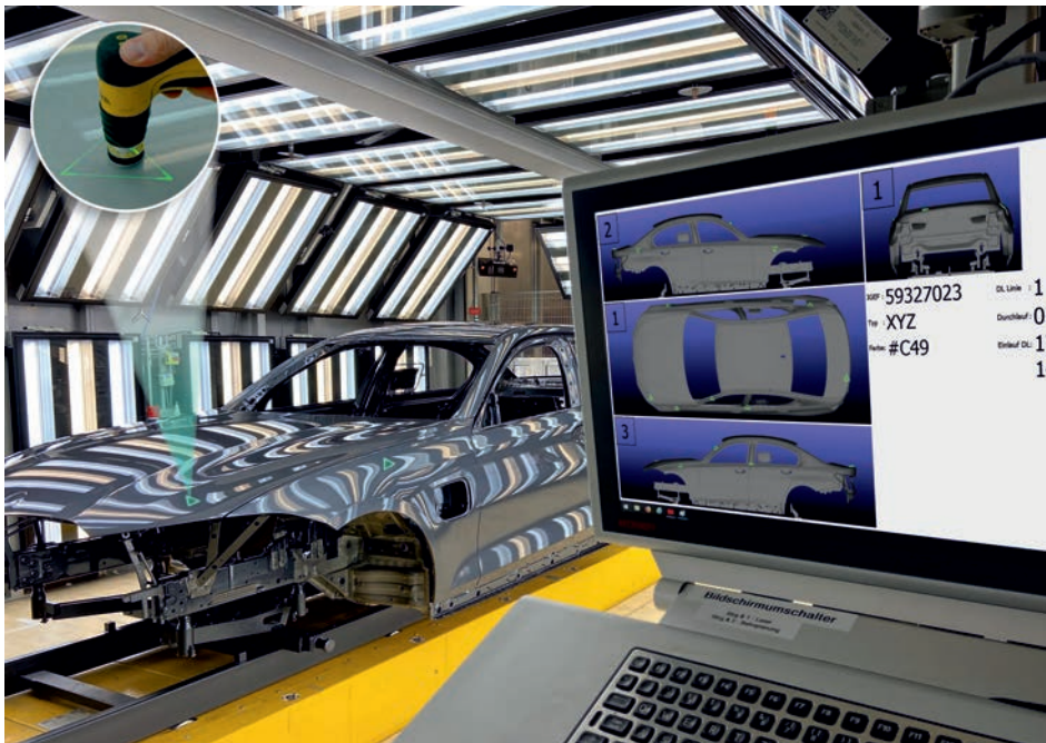
Figure 2. A butterfly view of the car body improves the overview. © Extend3D
